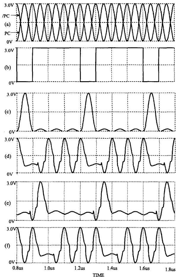
Fig. 3. Waveforms obtained from HSPICE simulations of a 4-stage pipeline of PAL inverters. (a) power clock (PC and /PC), (b) input of 1 st stage, (c) output of 1 st stage, (d) output of 2 nd stage, (e) output of 3 rd stage, and (f) output of 4 th stage.
