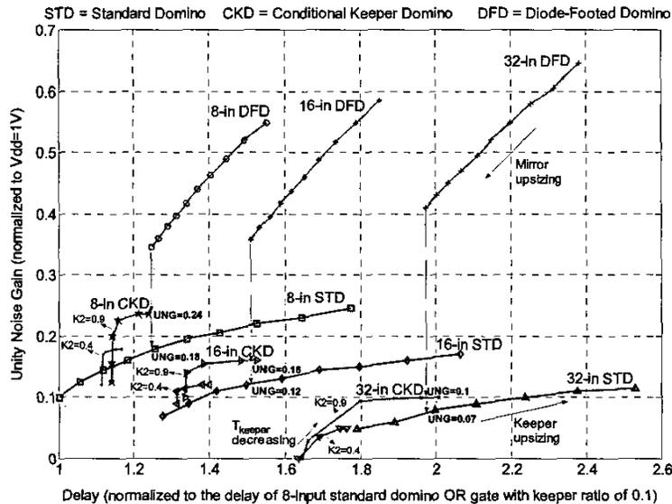
Fig. 6. UNG-delay curves for wide dynamic OR gates.
