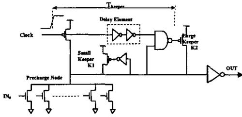
Fig. 2. Wide domino OR gate using conditional-keeper technique [9].
