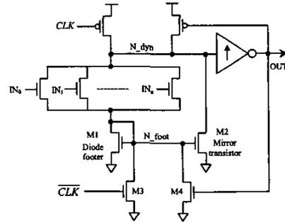
Fig. 4. Wide OR gate using diode-footed domino technique.
