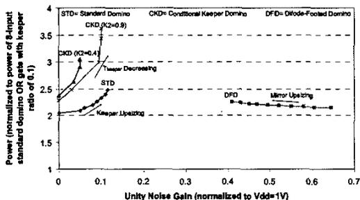
**Fig. 7.** Power consumption versus UNG for 32-input standard, conditional-keeper, and diode-footed domino OR gates.
