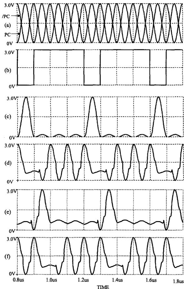
Fig. 3. Waveforms obtained from HSPICE simulations of a 4-stage pipeline of PAL inverters. (a) power clock (PC and /PC), (b) input of 1<sup>st</sup> stage, (c) output of 1<sup>st</sup> stage, (d) output of 2<sup>nd</sup> stage, (e) output of 3<sup>rd</sup> stage, and (f) output of 4<sup>th</sup> stage.
